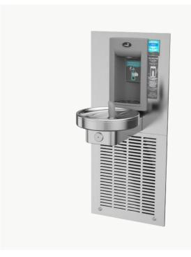
This wall recessed hydration station combo has two activation methods. The bottle filler includes an electronic sensor for a contactless (touch free) activation and a 30 second shut off timer. The radii drinking fountain is activated via a vandal-resistant push-button.
